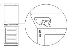
**13.** Carefully slide the fridge compartment door onto the top bearing pivot and close.
